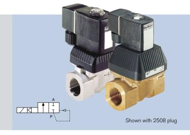
Soft-coupled, normally closed solenoid valve with a plunger piloted rolling diaphragm seal for neutral liquids to 194 °F. Its high flow waterhammer-free design allows switching from 0 PSI. For complete opening, a differential pressure of at least 1.5 PSI is required.
