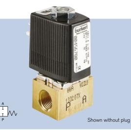
Direct-acting miniature solenoid valve which is plunger operated for neutral gases, liquids and technical vacuum. Available in standalone or manifold mount versions, there is also an "analysis" version which is manufactured under cleanroom conditions.
