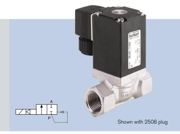
One of the ever reliable workhorses of the Bürkert solenoid range this hard-coupled solenoid valve with plunger piloted rugged diaphragm seal is perfect for vacuum, neutral gases and liquids. Its durable heavy duty construction is available in brass and stainless steel with a range of diaphragm and seal materials.
