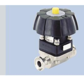
Hand operated diaphragm valve designed specifically for 3A / FDA compliant bioprocessing tasks. The forged 316L stainless steel body can be delivered with your specific surface finish with a range of diaphragm materials to suit positive control of ultra-pure, abrasive and aggressive fluids. The diaphragm type valve is preferred in these applications due to its favorable flow characteristics, its cleanability and its zero dead volume design.
