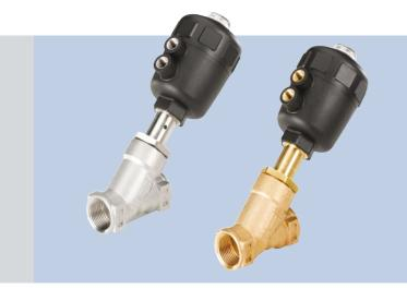
Bürkert's classic angle seat valve for on-off steam applications. Depended upon around the globe for unsurpassed lifetime. Its closed configuration with overseat flow for steam and gases these valves exhibit live loaded packing, N-seal piston actuator all in a rugged compact envelope.
