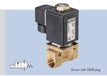
High performance plunger operated, direct-acting solenoid valve with integrated metallic body seal and wear resistant stainless steel seat. Three way (Type 0355), high pressure (1470 PSI), and high temperature (482 °F) versions are also available.
