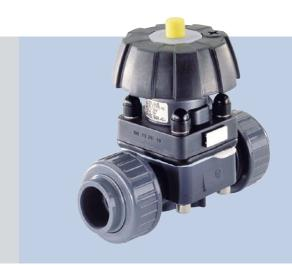
Hand operated diaphragm valve for aggressive chemicals. Provides long service life even with polluted, dirty or high viscosity fluids. The diaphragm between the actuator and body hermetically isolates the fluid from the actuator and provides a strong seal over the valve seat. The manual nature of the operator means that the valve can be used for shut-off and for flow control.
