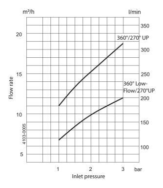
For Clip-on models, the flow rate is increased by approx. 1.5 m<sup>3</sup>/h
